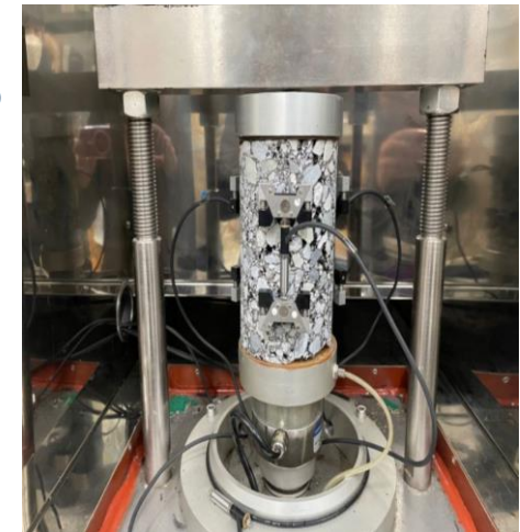
Figure 11: Fatigue results of AC 32 dense base 40/60
