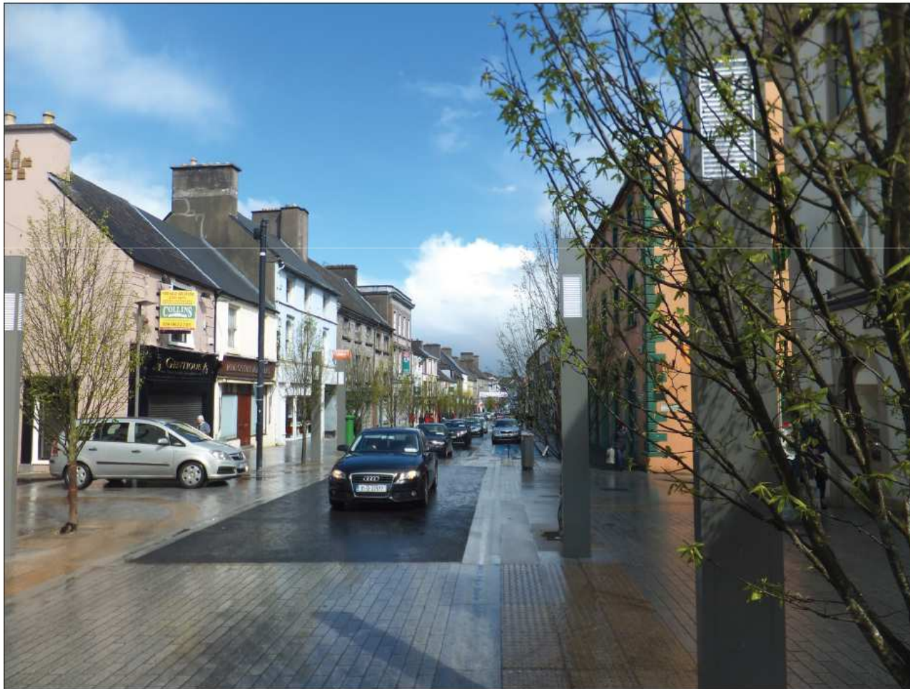
Figure 2. Self-regulating junction using contrasting surface materials
