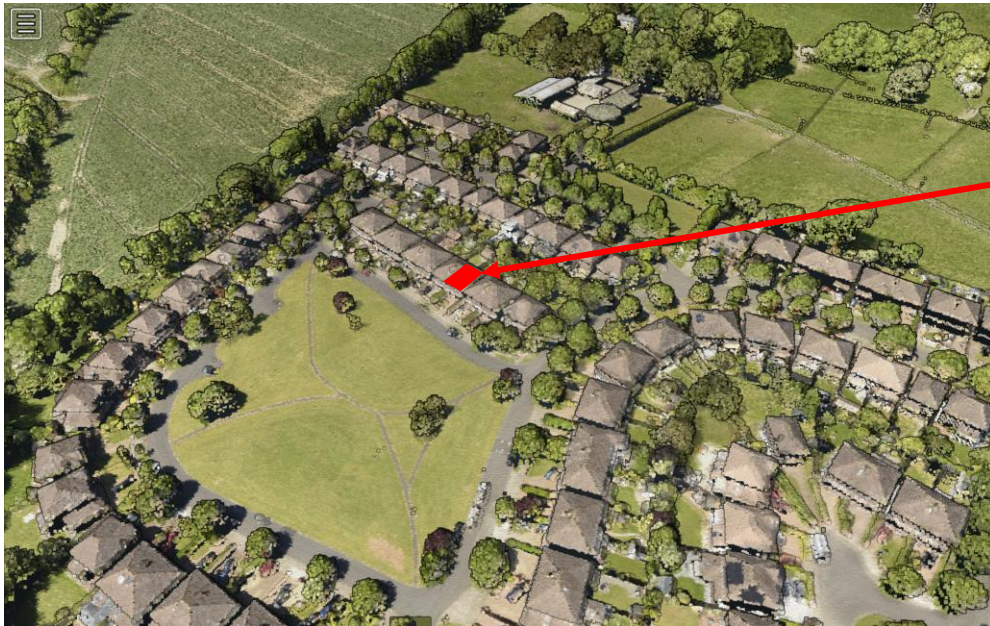
LiDAR data to determine roof area & slope
