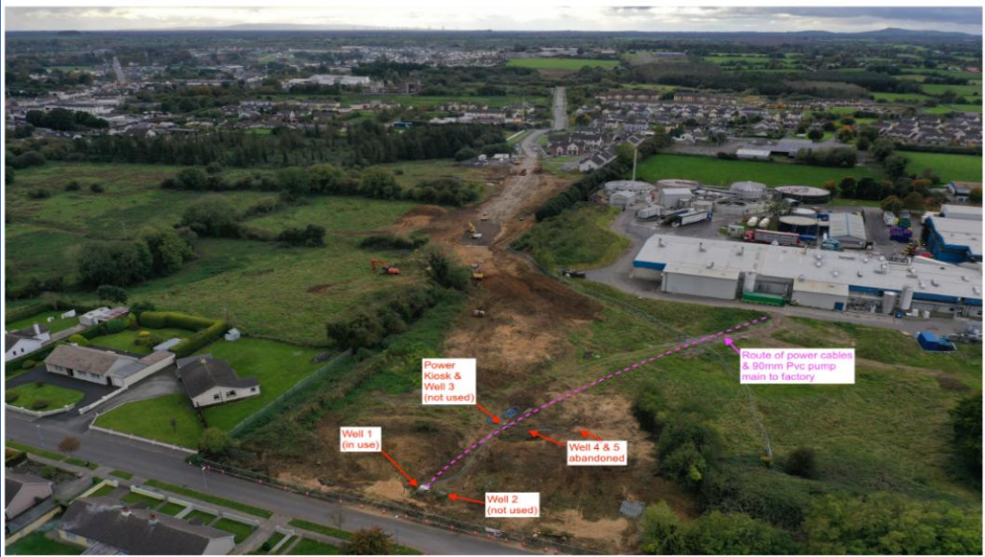
Well Locations relative to Rosderra Plant
